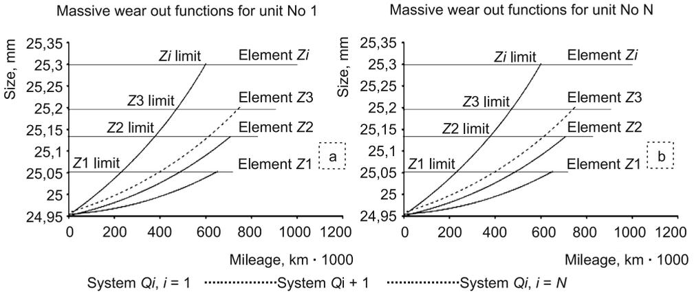
Fig. 3. Massive of modeled wear out functions
