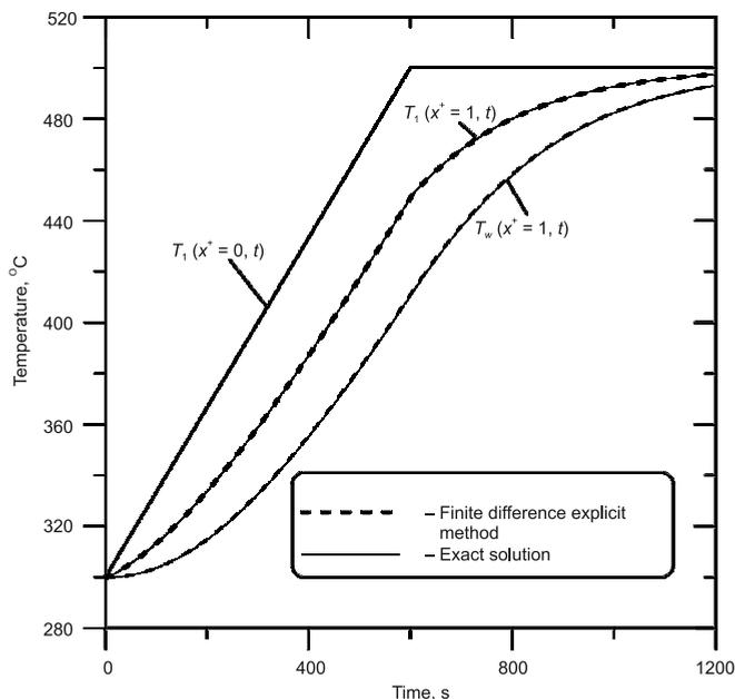
Fig. 3. Comparison of fluid and pipeline wall temperature at the pipeline outlet ( $x^+ = 1$ );
