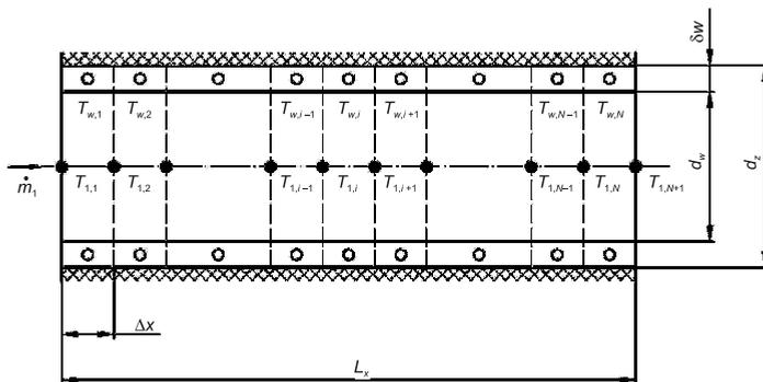
Fig. 2. Finite difference grid for fluid and pipe wall; • – fluid, o – pipeline wall
