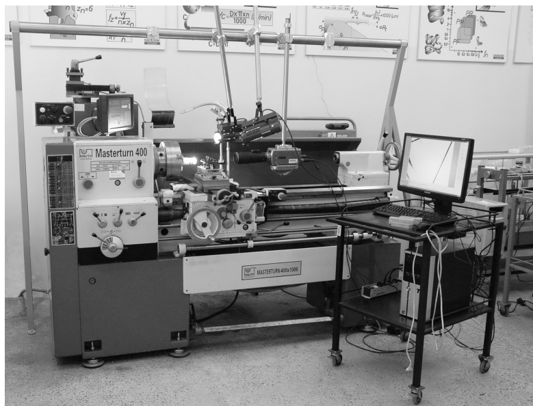
Fig. 3. Test stand for recording phenomena in cutting zone in turning
