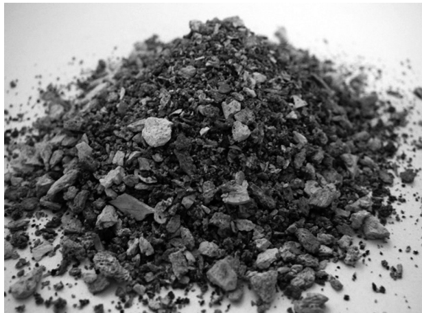
Fig. 1. The ash obtained from burning of MBM at 750°C
