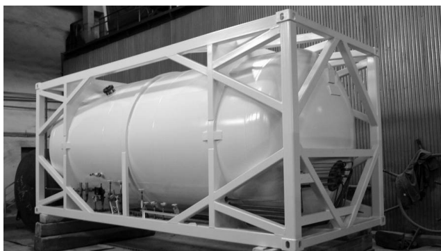
Fig. 15. 20-foot container for transporting cryogenic liquids introduced into production in Chemet company
