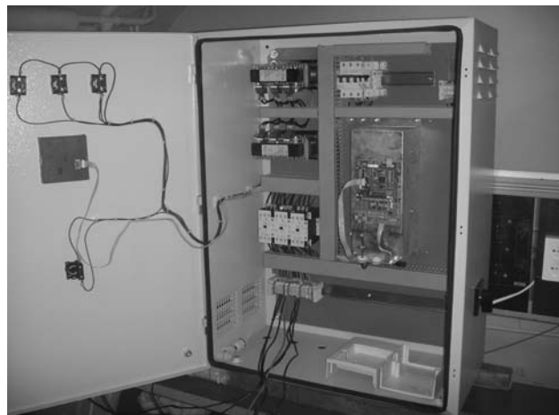
Fig. 13. Laboratory model of a back to back converter
