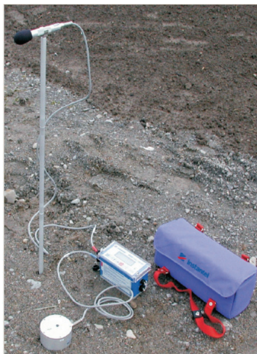
Rys 3. Rejestrator 4-kanalowy (drgania XYZ + hałas) Fig 3. 4-channel recording device (3D vibration + noise)
