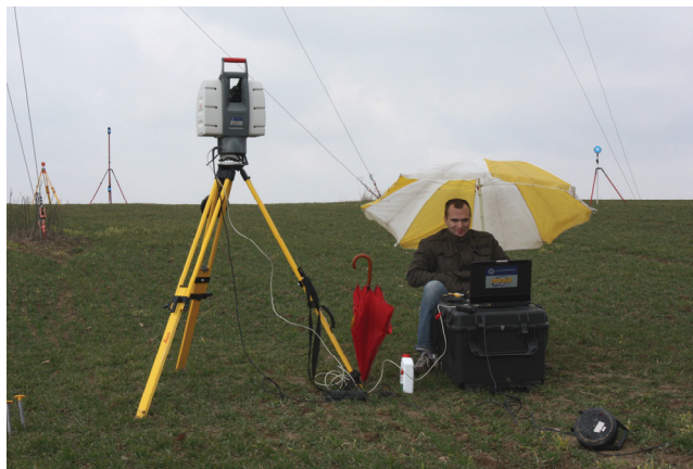
Rys. 4. Pomiary instrumentem Leica ScanStation Fig. 4. Measurements with Leica ScanStation
