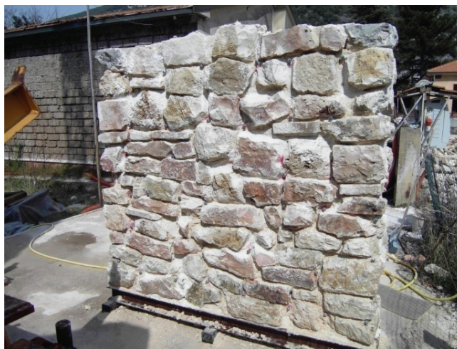
Fig. 6. The second panel subjected to flexural tests Rys. 6. Druga płyta poddana próbie zginania
