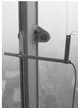
Photo 5. Probes for air flow velocity measurement
