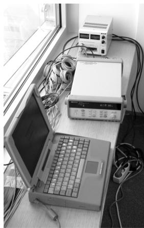
Photo 1. Data acquisition switch unit
