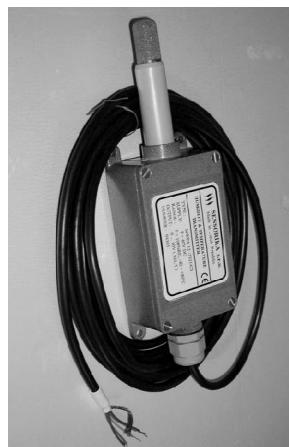
Photo 2. Temperature and humidity convertor
