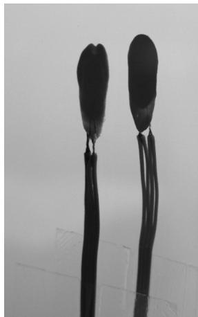
Photo. 4. Probes for surface temperature measurement
