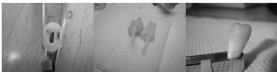
Fig. 1. Subsequent stages of premolar tooth sample preparation with glass fiber post reinforcement.
