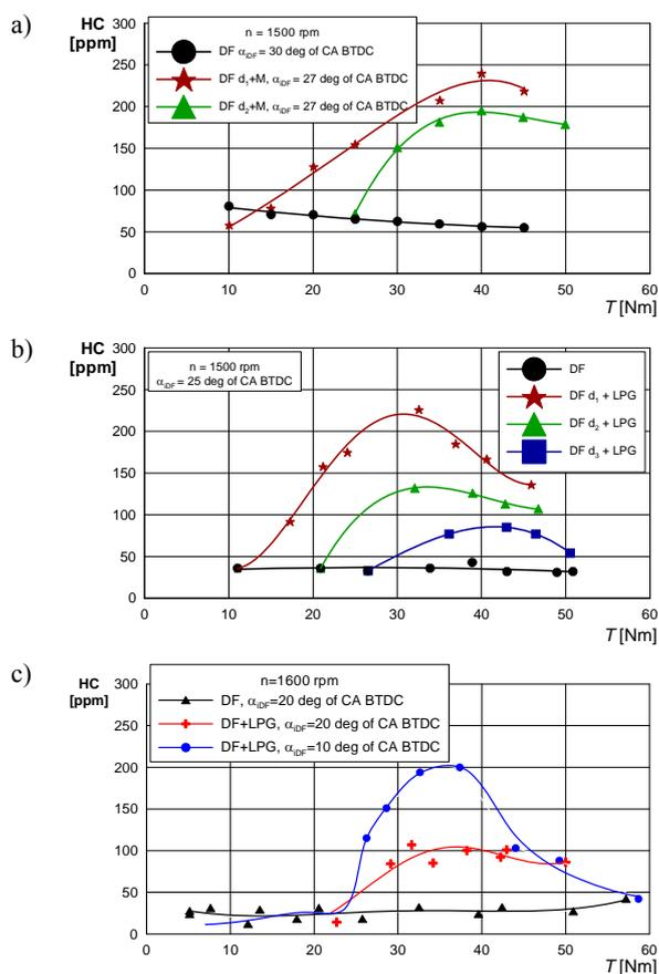
Fig. 4. Comparison of HC emissions for fuelling modes: a), b) and c) (described in chapter 1)
