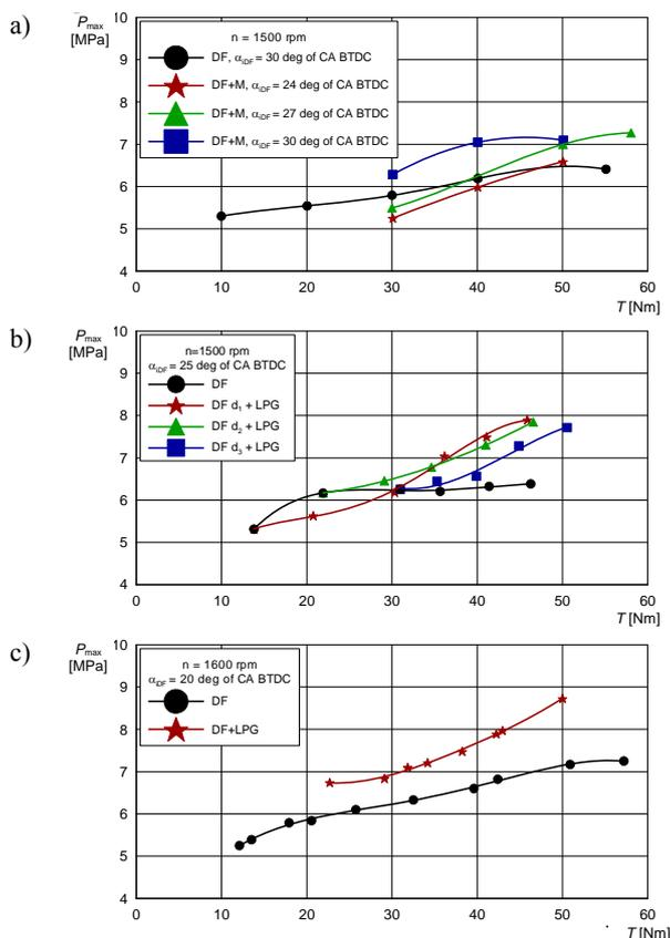
Fig. 8. Variability characteristics of maximum combustion pressure  $P_{\max} = f(M)$  for various injection timings of the pilot fuel and for fuelling modes: a), b) and c) (described in chapter 1)
