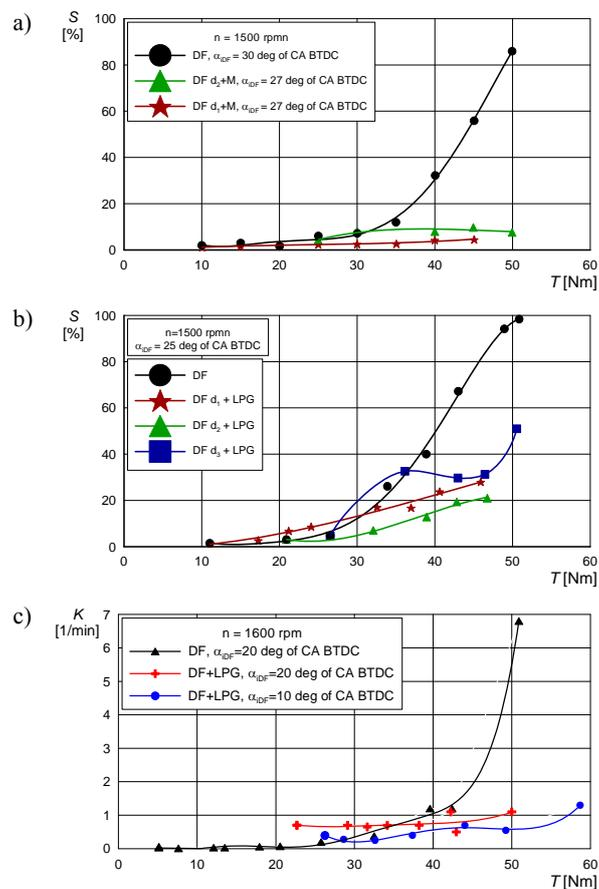
Fig. 6. Comparison of smoke level characteristics for fuelling modes: a), b) and c) (described in chapter 1)
