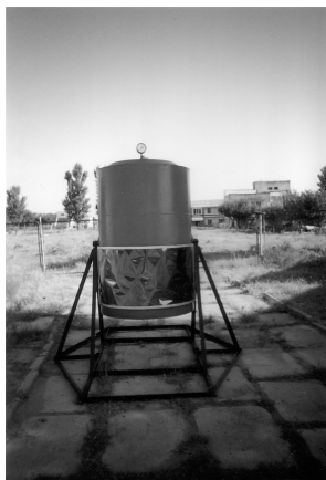
Fig. 1. Operative biological unit for utilization of organic wastes with usage of solar energy and heat accumulators based on phase transition materials
