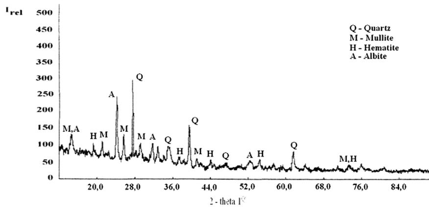
Fig. 1. XRD pattern of starting coal fly ash
