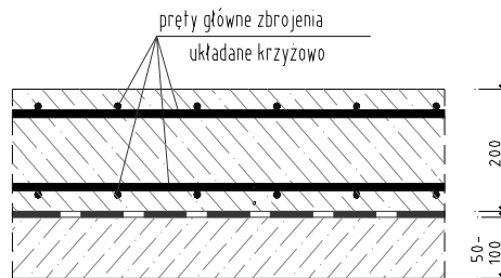
Fig. 1. The floor on the ground (layer arrangement)
