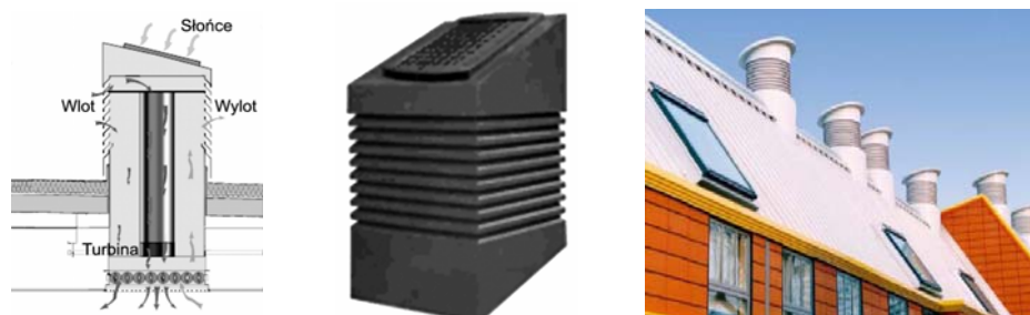
Ryc. 2. Centrala dachowa – schemat działania. Addey & Stanhope School w Deptford Fig. 2. Roof ventilation box – diagram of working. Addey & Stanhope School w Deptford
