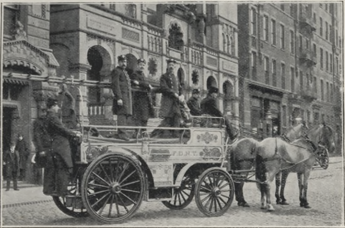
HOSE WAGON, CARRYING SCALING LADDERS.
