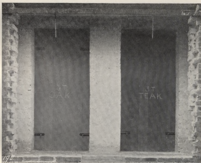
Fig. G. VIEW OF DOORS BEFORE COMMENCEMENT OF TEST.
