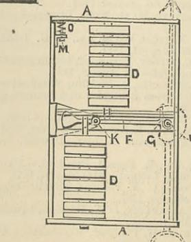
dications, of the combination of two groups of barometric chambers D independent of each other, and acting on each side of the pivot K of a lever F;
