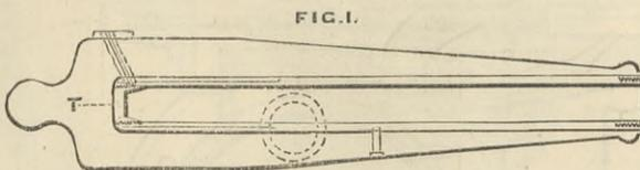
see BB and CC Fig. 3 and Fig. 4. The cup which formed the bottom of the bore was, of course, blown out to the rear with the breech, the coils into which it was screwed being unwound, as shown in Fig. 2 and Fig. 4. The coils do not appear to have been rent, they seem to have held well together, vide Fig. 4. The writer of the Spanish report considered that the longitudinal work was equally divided between the projectile and portion of
