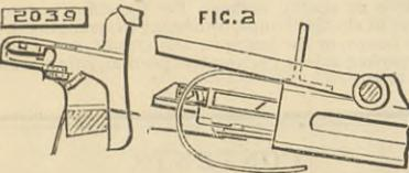
pinion on this axle lifts round its driving cog wheel R, hanging on the centre by the short cranks, thus allowing the intermittent revolving axle to rise in case the arms K should strike the ground while revolving. Fig. 1 is a side elevation of the apparatus, and Fig. 2 an elevation partly in section showing the binding mechanism.
