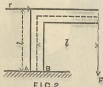
To make the above formulæ applicable to an unsymmetrical cross-section, we have only to express that the two forces,  $W_1$  and  $W_2$ , are to be considered as applied at a point in the centre of gravity of the section, and we then obtain—
