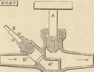
valve, such as B B', the stem of such valve being placed on the upper side or upon the same side as the stem of the ordinary valve A A' of such taps or valves, in order to afford greater convenience for regulating or cutting off the flow of fluids through such taps or valves.
