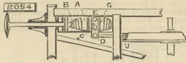
cylinder E, behind which is a spring G. The arm D is connected to brake block J. The invention relates, Secondly, to the application of a toothed disc to the wheel axle, and a metallic piece operated by cord or lever is capable of engaging with the teeth so as to stop the rotation of the wheel.
