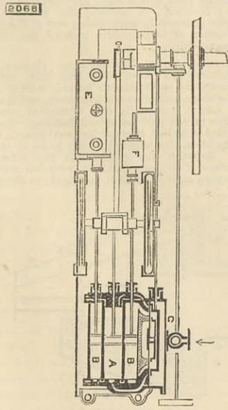
condenser E is operated by one of the low-pressure piston-rods, and the force pump F is worked by the other. The supply valves of the low-pressure cylinder also serve as the exhaust valves for the high-pressure cylinder.
