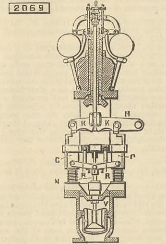
sion valve, and it consists of a lever H, to the end of which the eccentric rod is attached. To the lever two bell-crank levers K are pivotted, their horizontal arms being jointed to the sliding governor rod by means of links, while their vertical arms act on sliding pieces G connected by levers R to valve rod N. Springs act on the pieces G so as to close valve V when the crank levers K cease to act on them.
