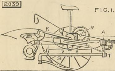
teeth of this rake run underneath the sheaf to be bound, and the rake meets all irregularities of the ground by working or lifting on the forward centres T. An intermittent revolving axle passing across or near the centre lengthwise of the frame A carries projecting arms K of suitable length, which lift the corn to be bound up the trailing rake S about to level with the top of the frame A. This intermittent revolving axle may be carried at each end by short cranks. A
