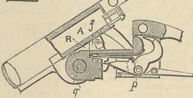
underneath and in the hinge lump R turning upon the centre pin q the ejectors are pivoted, then by making use of a shorter breech action the centres q c p are so arranged that the barrels A drop of their own weight, and without any assistance from the breech action, lever, or bolts in connection therewith. Other improvements are shown and described.
