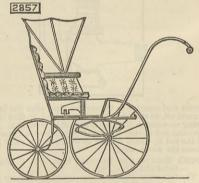
to shift its position and thereby shelter the occupant from wind or rain. An arm is fitted to the movable part and carries a roller resting on the bottom of the body, so as to relieve the pivot from undue strain.
