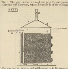
the gas becoming charged with gasoline in its passage and finally passes out at G.
