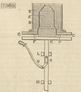
pattern, and venting the exterior unrammed sand<sup> $\blacksquare$ </sup> The drawing shows a vertical section of a machine and flask, with the pattern and sand contained therein. A is the pattern, B the metallic flask which surrounds it having its side equidistant at all points from the pattern A, and having grooves or channels formed with open sides towards the pattern. E is the sand mixed with an agglutinating fluid; F, tapering venting
