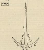
quantity of the strain from the pin. A hole E is made in the crown at right angles to the axis of the flukes when open, through which to place a buoy rope. The connecting pins of the flukes are preferably screwed. When folded for stowing the flukes lie very close against the shank.
