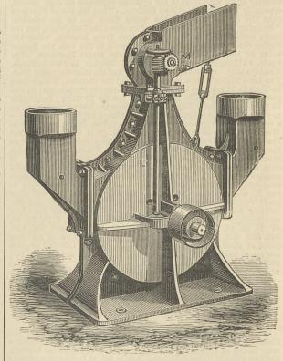
for the same reason, immediately returned. Thus it is with great force struck to and fro from arm to arm until as fine as required. There is therefore no grinding action, the crushing being done
