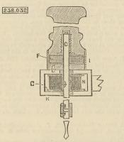
(2) In a drill stock, the combination, with the handle, having socket and bearing, and with the shank C, that carries the drill, of the coiled spring F, the spool G, the ribbon H, the guide K, and the case I, substantially as herein shown and described, whereby the drill will be rotated by alternately drawing upon and slackening the ribbon, as set forth.
