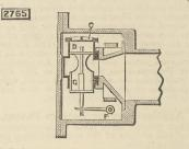
structed of two disc valves C. These valves work in cylindrical cases D, and are in contact with levers E, which are actuated by an ordinary governor moving the spindle F, so that the said disc valves act as throttle valves, one for each end of the cylinder.
