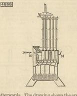
ately afterwards. The drawing shows the arrangement of the moulds. Each consists of a case or mould carrier M of copper, in the middle of which is fixed, by screwing or otherwise, a tin or pewter mould. Into the space surrounding the mould cold or hot water may be admitted at will by pipes arranged at top and bottom of each mould case.
