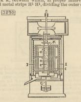
ference into alternate large and small spaces. In each of the small spaces is placed a brush L, and in each of the larger spaces is placed a series of vertical rods 1<sup>1</sup> 1<sup>1</sup>. Each series of these rods is placed upon the arc of a circle excentric to a circle having the shaft C as a centre; or in other words, these rods in each series form an inclined rod beater, by which the wheat is carried up an incline to the face of the adjacent brush.
