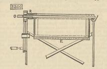
shown in the drawing. This apparatus consists of a toothed pinion R driven by a spur wheel, and having a hollow boss connected with the vessel containing the tempering liquid. To this pinion the cannon is connected so as to revolve with it, and the tempering liquid passes through its bore. Beneath the cannon are fire bars E, upon which a charcoal fire is kept burning during the operation.
