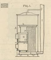
which are placed closely together, sufficient space being left between them for the circulation of water. At the front part of the boiler the chambers D E are connected by partitions G that form the fire-box H. Is a pipe for carrying off the steam and products of combustion. In Fig. 2, A is a wheel carried by a shaft supported in bearings. The rim of the wheel is
