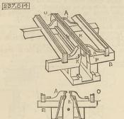
A, provided with lugs K, in combination with the angle iron stringer X, substantially as and for the purpose described.
