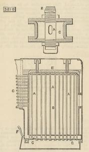
tube-plate there is a double row of tubes, so as to more effectually intercept and absorb the heat of the gases before passing into the boiler tubes G. The top ends of the tubes A are tapered and screw-threaded as shown at K in the second figure, and their bottom ends are screwed where they pass through the top and bottom plates of tank C, lock nuts being fitted over their lower ends. The part of the tube within the tank is perforated to allow of the free circulation of water through them.
