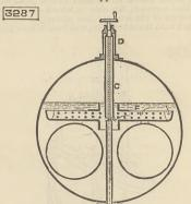
The hood-pipe is shown to be raised and lowered by means of a quick-threaded screwed rod rotated by a wheel and handle. F F are scun troughs extending across the boiler and resting on the flues, and extend-ing also lengthway of the boiler at each side for any desired extent.
