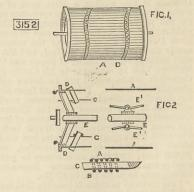
for actuating wires. A are the screen wires, every alternate one being fixed, and the remainder loose; B corrugations which alter the mesh, same being arranged in a screw-shape round the screen; C double internal coil for moving corrugations; D double external coil; E boss on hollow shaft of the screen, on which are cast lugs for the attachment of the wires El which move the coil C.
