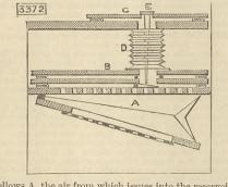
bellows A, the air from which issues into the reservoir B of the pipe organ. The reservoir C of the reed harmonium communicates with B by a throat D which allows the air to enter C by means of a guide E fixed to the upper part of C.
