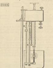
by the drawings. The action of the carbons is regulated by an electro-magnet, which with a varying
