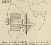
such short circuit entirely upon movement in one direction and intermittently breaking it upon move-ment in the other direction, substantially as set forth, (2) The combination of a driving shaft of a magneto-electric machine, a sleeve mounted thereon in such manner as to have a determinate longitudinal move-ment thereon, and a circuit breaker automatically operated by such sleeve, to break a circuit entirely during movement in one direction and intermittently
