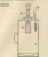
not easily acted on by the acid, by which means the acid cannot be made to get out by shaking. Over the mouth of the bottle is arranged a punch 16, by means of which the wax can be perforated, when the bottle is turned over, allowing the acid to mix with the carbonate solution; or the bottle may be inverted and the punch arranged beneath it, in which case the acid escapes at once without requiring the bottle to be turned over.
