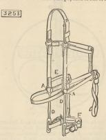
a plate F which is connected to the lower end of the bars D. The plate F has in front a number of spikes covered by a spring plate, so that the spikes will not enter the animal unless considerable pressure is availed
