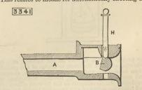
coupling of two carriages by moving them towards each other. The lower inner surface of the draw-bar A is inclined, and its upper interior surface is recessed and contains a pendant block B, which serves to
