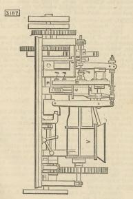
fitted, which dies can be changed to suit form and thickness required, whether front bricks, dust bricks, or quarries. A is the pug mill; B is the disc or mould to receive the largest sizes of dies the machine is capable of filling; C is part of the delivery apparatus which is worked from a cam on shaft E; D is a table on to which the bricks or tiles are delivered; F F are piston stalks in the moulds against which the press levers act when pressing.
