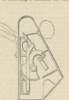
corn or other cut crops to a self-delivery reaper, and consists mainly in fixing the binder in the position ordinarily occupied by the table or platform of a reaper, said table or platform having been removed, so that the corn when cut falls direct upon the platform of said binder, instead of having to gather the corn when delivering reaper.
