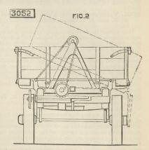
engine. Fig. 2 shows a wagon to be tipped by the tractive power of the engine drawing it. The body is placed low, and is jointed to the bed, so as to tip by means of a windlass arrangement, the pull of the engine causing a rope to be drawn off from a wheel or drum, thereby turning an axis and causing a chain attached to the body to be wound upon a barrel. Another arrangement consists in the use of an hydraulic jack.
