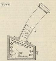
prevents the transmission of other sounds than those of the speaker's voice. Various modifications of the above form of speaking-tube are described and illus-trated. The figure shows the ordinary form adopted by the inventor. The inside of the tube is lined with soft stuff to modify harsh tones, and a tube leads off the condensed breath.
