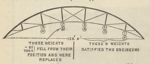
The total weight applied..... Deduct weight of sheets, glass, &c., which were not on at the time of testing 48 tons. 5 ,,
