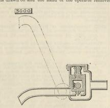
from the spindle or handle which opens the water-way, it becomes immediately closed, and the flow of water or other fluid at once stopped. The drawing shows a longitudinal sectional elevation of the tap.
