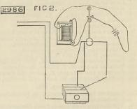
connected by conductors, and a commutator. The latter consists of three metal plates insulated from each other, and connected up as shown in the diagram, Fig. 2. Holes run through these plates,
