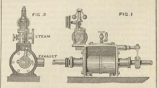
The cylinder is divided lengthways by a diaphragm, two piston cams D being feather keyed on the shaftS, one on each side of the diaphragm, and rotating in the direction of the arrow. These pistons are placed on the shaft in opposite positions to each other, by which arrangement the engine is perfectly balanced, and when the steam is exerting full power upon the one, the other is open to the exhaust; nearly equal pressure is maintained throughout the revolu-
