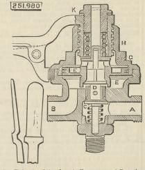
piston E, having lateral ports E, escape port G, springs C and H, handle K, and screw plug K, substantially as set forth.
