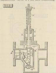
sliding drum and the spindle, the stuffing-box D. The exterior and adjusting arrangement consists of the bridge DI, the stop nuts below the bridge E, the spiral spring F, the washer and thumb-screw G.
