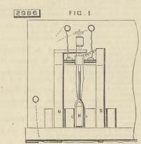
the other, making contact by means of platinum studs on it, with other fixed studs on either side, and so causing a signal to be operated indicating the subscriber who calls. To effect communication between two subscribers, the inventor uses two keys
