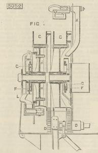
boiler, and driven by pinions D on an upright shaft. The coiling cams F are placed upon the axis above
