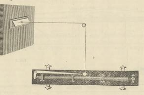
I have experimented with strips of different metals like those recommended by Dr. Ure, similar to the compensation balance wheels of a watch, and also to the metallic fire electrical alarms, but no power can be obtained out of such contrivances that will be serviceable for ventilating. I shall be glad to give your correspon-dent particulars of my experiments, which would occupy a great amount of your space and more of my time than I can afford just at present. Albion Works, Salford Manchester
