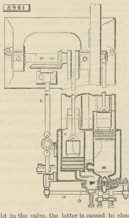
the light in the valve, the latter is caused to close a little before the piston in the compression pump has completed its stroke, thereby increasing the pressure of the remaining gases, from which source the light gets its supply. The opening and closing of the gas inlet valve is regulated by means of an ordinary governor and a tapered or stepped cam.
