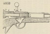
ing trigger F by means of two side lugs G that pass through corresponding slots in the trigger block F, so that if the latter is then turned partly round on the striker bolt it is held on the latter between the said lugs, and a shoulder formed thereon at a short distance from the lugs. Other improvements are described.
