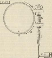
rubber or other material to give the necessary pres-sure on the warp beam. To the heop are attached angle pieces C with a spring E between them, adjust-able by means of nuits. To the bottom angle piece is attached a spring I, also adjustable by the screwed rod K
