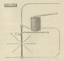
magnet opposed in their action, the latter being located in a shunt around the arc, substantially as set forth.
