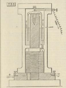
measured circulates through the magnet and the moving conductor, and as the force required to move any object through a liquid is proportional to the square of the speed, it follows that the number of totations of the conductor will be proportional to the current to be measured. The registering part of the apparatus may be independent of the above, and con-sists of an electric bell, and arranged with a train of wheels. Each pulsation of the armature registers permanently. permanently.
