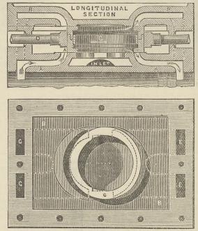
VALVE AND UNDERSIDE OF COVER IN PLAN
