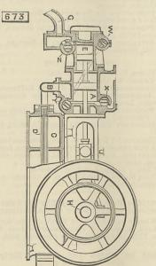
pipes D. Behind pump A is the expansion cylinder E which receives air from space C through valve W, and discharges it when expanded through valve Z, the air passing by pipe G to the place where it is to be employed. The valves X Y, W, and Z are all worked from excentrics on the shaft H driven by a suitable meter. motor
