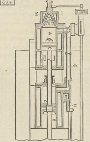
fitted with a valve H worked from the crank shaft. A charge being admitted to one cylinder is thus caused to exert a corresponding force on both pistons at the same time. M is the valve to admit the charge to cylinder A, and over it works an ignition slide. 632.
