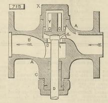
the valve Y, the seat D of which is formed in the body of the cock, and which is kept closed by the pressure of the water. The operating rod forces the valve from its seat when required to be opened, and when the pressure is removed the valve closes. Small holes O allow the fluid to pass under the valve so as to facili-tate its moving.
