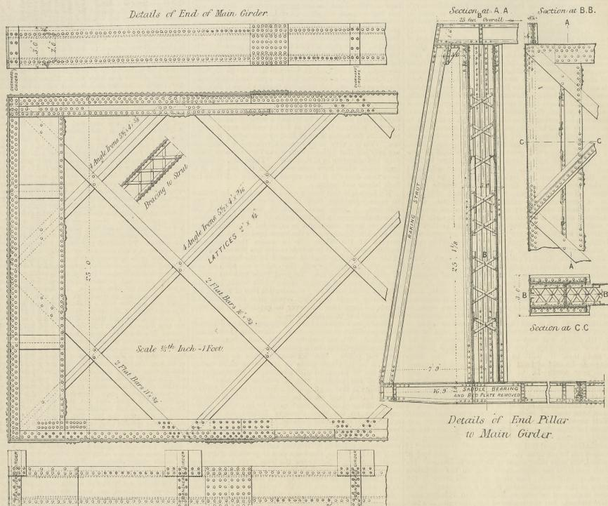
In our impressions of the 18th and 25th ult. we have given a perspective and detail drawing of this bridge, which has been designed to carry the Brazilian Imperial Central Bahia Railway over the river Paraguassa, between Chachocira and Sao Felix, and at the same time to act as a road and foot bridge.
