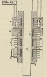
forming parts of discs, provided with pins E, adapted to form electrical contacts with the segments of the wheel Al. (2) The combination of a commutator wheel Al, having insulated segments and spring fingers El, with a commutator wheel, A, having seg-ments secured to or forming parts of discs, provided with pins E, to come into contact with the fingers E<sup>1</sup>.
