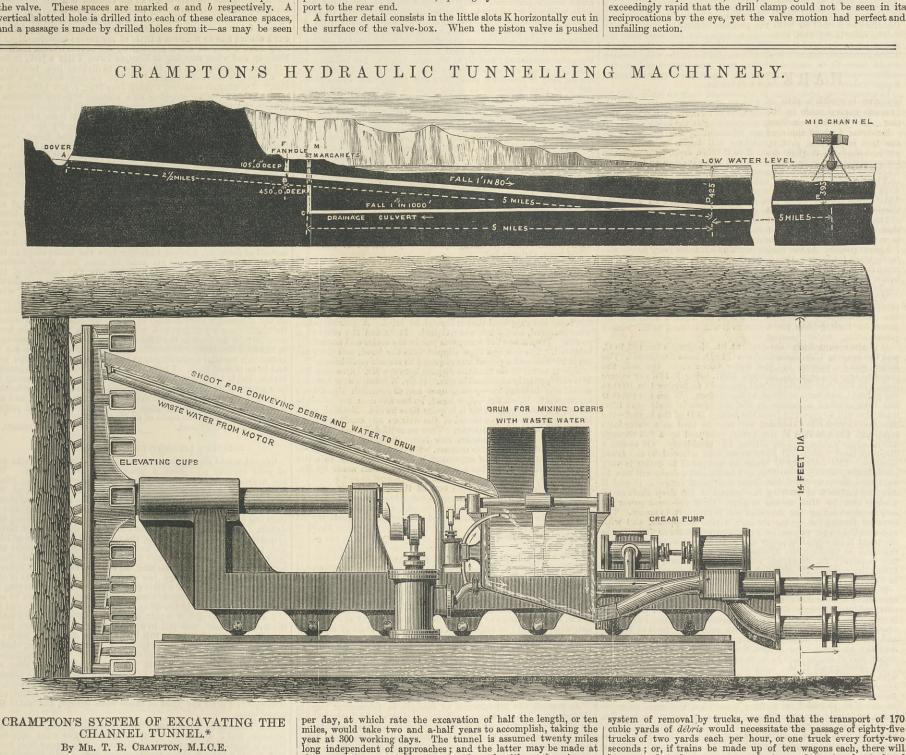
It is assumed, to avoid complications in this statement, that there underlies the bed of the Channel between Dover and Calais an uniform stratum of grey chalk—impervious to water and so soft that it can easily be cut by ordinary cutting tools or chisels. Practical trials made with machines many years since and also more recently have established the fact that a rate of advance may be easily maintained of one yard per hour, or twenty-four yards
