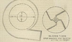
of the hand-wheel. The fan case was 6.5in. wide inside, and the wood tube to the rick was 6.5in. by 7in. The engravings show the form of the fan and the arrangement. Mr. Pratt also showed the same fan driven by a strap, and the whole arranged with a small horse gear on one frame.
