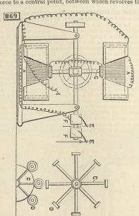
wheel C carrying coils D. The brushes E E collect from F F, and convey the current to the lamp or amps
