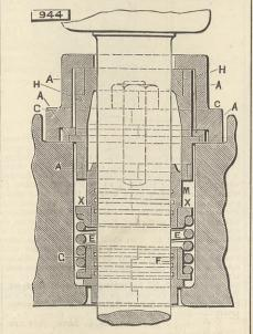
halves, and holding it in place by the rings A, the cap C securing it in position. M is the follower, also in two pieces held together by ring X at one end, and by passing into the packing receptacle at the other, F is
