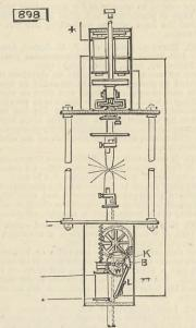
an insulated boss B, a lifting pin, a contact lever L, and spring K. Other modifications are described, as with a definite feed to one carbon, while the other is regulated by a solenoid, &c.
