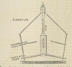
The application of an exhaust ventilator exhibited by Messrs. C. Kite and Co. is shown in the annexed diagrams. To this we
