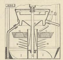
for the water jet, placed in opposite directions, and through either of which the water can be directed. A water-spray apparatus H is combined with the venti-lating fan I on shaft G, for the purpose of moistening and purifying the air, the water passing from the turbine casing into the spray apparatus by funnel O. A disinfecting apparatus S may also be secured to shaft G, and consists of a perforated trough contain-ing sponge, to which a disinfecting fluid is supplied and thrown out in a spray.
