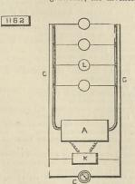
method illustrated in the accompanying diagram. It consists in operating the regulator by a circuit taken across the main lines at a point where their influence, as a varying factor in the resistance, will be nearly or quite eliminated. A is the generator, L L lamps, C C regulator circuit, R regulator, and G galvanometer.
