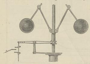
method of attachment. If the engine exceeds its ordinary speed the governor balls fly outward, and the finger A presses on the plate B. On the other hand, if the belt or gearing used to drive the governor gives way, the balls at once fall, and the finger C presses on the plate B. In either case the circuit of the electric current is closed, and the stop valve on the engine screwed down.
