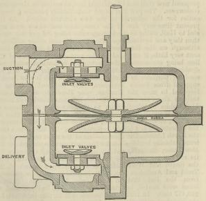
by alternately raising or depressing the india-rubber diaphragm. The general arrangement can be understood from the engraving.
