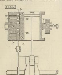
what C-shaped, and provided with steam ports J and exhaust ports K, and it is worked from an excentric on main shaft. 1150. Holding and Adjusting Lawn Tennis Nets
