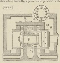
two compression rings M and packing rings N sepa-rated by a follower P, the outer rings M being fitted to receive steam from the chest, and the inner rings from the cylinder.
