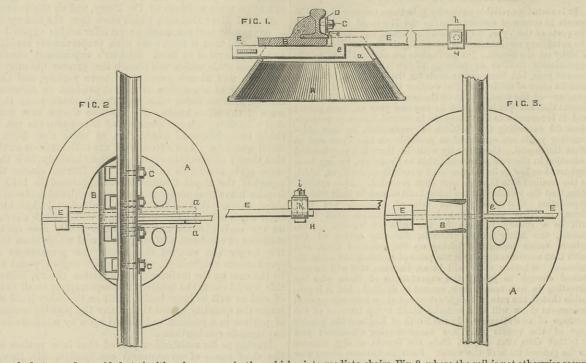
in the top table and partly in the sides of the pot sleeper Å, and its straight extremity passes close under the top table of the sleeper, and is secured at the opposite side by a key E. The
