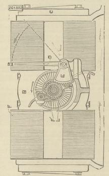
holder H, brushes carried thereby, cog wheel F<sup>1</sup>, of the toothed segment E and lever D, these parts being constructed and combined in substantially the manner set forth. (3) The combination, of brush holder H, brushes carried thereby, cog wheel F<sup>1</sup>, toothed seg-ment E, lever D, and resistance coils R, said coils being placed as described, and arranged to be thrown in and out of circuit with the brushes by the move-ment across them of the lever D as described.
