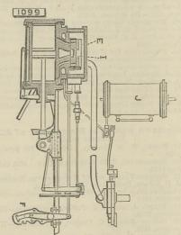
relatively to the piston, whereby an earlier and a greater variation of cut-off, with better distribution, are effected. Another feature relates to the better lubrication of valves which are held to their seats by pressure of the motive agent on their backs, and it consists in supplying the lubricant to the face of that valves from reservoir J, where the lubricant is main-tained under pressure.
