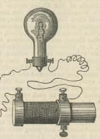
closed, so that there is contact between the coils. The circuit wires connect to the ends of the coil at the fixed and sliding collars. The resistance offered by the coil depends upon the length of the coiled portion opened by adjustment of the slide. The closed portion is short circuited, and allows the current to pass freely. This regulator may be used for electric currents generally, and is specially adapted for electric lamps. It is the invention of Mr. Patrick H. Fox, of New York city.
