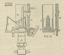
marker on the paper. A is the cylinder of the indicator, B the marker lever, C the rotary paper carrier, and P the parallel motion. To the base of drum C is fixed a cam E, which acts on a lever F, the outer end of which enters a groove in a vertical screw or rack X, and moves it upwards, and through a suit-able ratchet the marker will be intermittently raised at each stroke of the piston. Other improvements are described lescribed.
