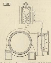
slide C works, such grooves communicating by means of a pipe F with a chamber E, containing fluid sub-jected to the pressure of the motive fluid, and also heated by a gas jet Y.
