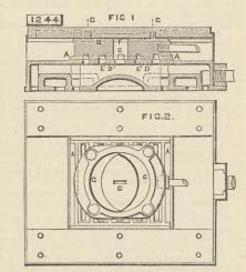
between the space F, enclosed by the ring G, and the interior or steam port space of the main slide in every position which the valves can be placed in by means of a hollow passage C through the cut-off from front to back, made long enough to overlap the bridges D between the steam spaces E as much as may be necessary. The ring G is carried in a groove in the back plate of the main slide, and is held in contact with the back of the cut-off by helical springs.
