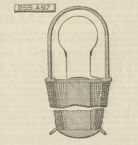
substantially as set forth. (2) The combination of a glass globe containing the light-giving part, an extension made integral therewith, and secondary coil supported at the interior of the extension and placed in circuit with the light-giving part, and of a primary coil arranged exterior to the globe and in inductive relation to the secondary coil, substantially as specified. 255,518. SPINDLE-STEP RAIL FOR SPINNING FRAMES Francis Leclère, Philadelphia, Pa.—Filed December
