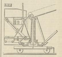
the working parts of any movable hydraulic crane to serve as a counterpoise to the load to be raised, without the aid of the usual tail-jib balance.
