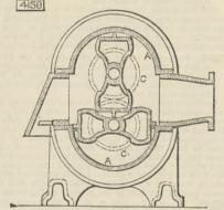
sists of two semi-cylindrical flanged shells A secured between end-plates, and in it the rotating abutments C are mounted one above the other, the form of which will be seen in the drawings. Means are provided to adjust the abutment shafts in case the bearings wear
