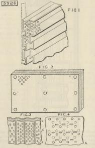
sheets, roughened, serrated, or indented, composed of lead, platinum, or carbon, upon, in, or against which plates spongy or finely divided lead or oxides, or other salts or compounds of lead, or other suitable substances or compounds, are, or may be, held. The figures show some forms adopted.
