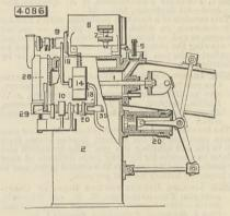
which it passes by valve 9 to the power end of the cylinder, the valve being operated by a cam 10 and lever, such cam also operating the gas admission valve 14 which is actuated or disengaged by the governor. The gas passes by pipe 18, and mixing with the air is conveyed by another pipe to the cylinder; 20 is the gas pump driven from the piston crosshead. The ignition slide 28 is driven from crank 29, and the cam 30 regulates the exhaust, both being fixed on shaft 35 driven from the crank shaft.
