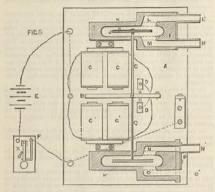
of the magnet C will cause air to be expelled from the air passages L and N, and at the same time to be sucked in by M and O, and vice versá.
