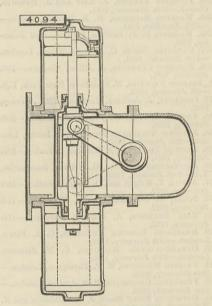
set of valves and with or without fixed pump barre covers, and containing the working gear for actuating the pistons. The drawing shows a longitudinal vertical section of one arrangement.
