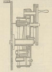
a spindle attachable to, or connectable directly with, the plate at the part to be cut out, the said spindle or upright forming the working centre of the machine and supporting or steadying the apparatus.
