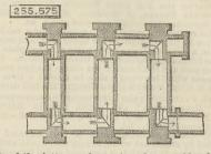
ends of the latter, and a series of removable plugs extending transversely through the longitudinal pipes at points opposite the ends of the transverse pipes, and constructed to direct the flow of beer from the longitudinal into the transverse pipes, all substantially in the manner and for the purposes set forth.
