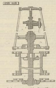
bar, a feed screw concentric therewith, a gear journalled upon a casing which is fitted to move with the boring bar longitudinally on the feed screw with-out rotating with the boring bar, a sectional or divided nut pivotted to said gear, and a clamp by which said nut may be made to either engage with or be removed from contact with the feed screw.
