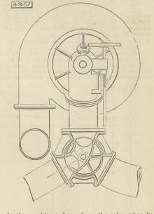
each other, and to wedge or force the valve when in its extreme positions against the inlet that is closed.
