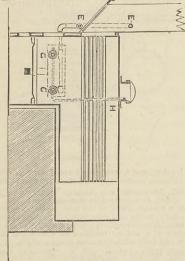
the stack through the pipes E E air and whatever the state through the pipes E E ar and whatever unconsumed smoke and gases may escape from the fire, and discharge same mingled with the jets of steam through the nozzles G G over the grate, hot air being also sucked out of air chambers and down through tubes in the same direction.
