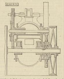
counter shaft having one end extended through and made vertically movable in a slot in the said plate, and a link connecting the counter shaft at this end to the axle, substantially as and for the purpose described.
