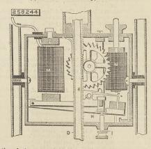
the electro-magnet N, forming part of a derived circuit, its armature N, a device for breaking and closing said circuit, the moving frame H, escapement G, escapement wheel E', pinion E, racked carbon-holder A, and means for allowing the armature to move a sufficient distance to insure the working of the
