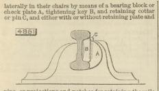
pins, or projections and notches for retaining the rails longitudinally at their end joints.
