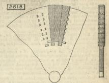
width will admit of; he then continues the winding through a series of holes pierced through the disc, or steps cut in the segments, in such manner that each successive turn is shorter than the one preceding it. In this manner he fills up the otherwise unoccupied triangles with winding in a series of turns arranged stepwise, as shown in the accompanying figure.
