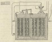
of a support or plate with a layer of porous active material applied thereto, composed of oxide of lead or its equivalent, mixed with fibre or filaments-in contradistinction to pulverised coke or sawdust-whereby the porous mass is bound together and held more securely to its support or plate. (4) The improved porous active composition for secondary batteries, consisting of a mixture of oxide of lead or its equiva-
