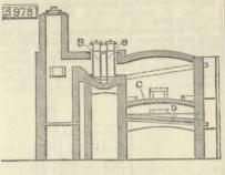
copper, tin, and zinc; and it consists, First, in form-ing the hearth C, on which the ore is first treated, with holes, through which the ore can fall as it is fused; Secondly, in causing the fused ore to fall on a solid bed D, beneath the perforated hearth C; Thirdly, in treating the oxides in reducing chambers B arranged so that there is a downward draught through the material.
