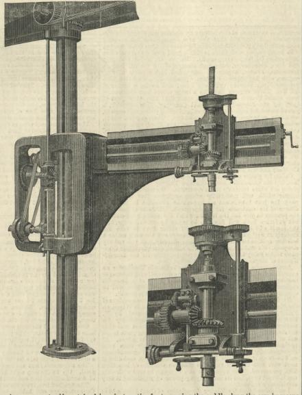
gearing, &c., are carried within the framing of the radial arm, forming a compact self-contained driving apparatus. The saddle on the radial arm is fitted with of a hand-wheel placed on the saddle within easy access of the the usual hand-feed and self-acting motions, and also with a conworkmen.
