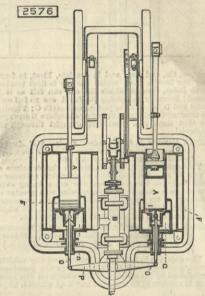
inlet valves I are carried in a cylindrical guide formed at the central part of the delivery valves, the stems of which are tubular to admit the air. The two inlet valves are coupled by links O and lever P. Springs are attached to the tubular stems of the delivery valves, so as to insure the proper closing of such valves before the pressure of the air is sufficient to effect this object.
