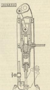
the working barrel, substantially as described. (2) The combination of a fixed discharge chamber, a pump barrel detachably connected thereto and sup-ported thereby, a valved piston, a piston-rod having half the cross sectional area of the piston, and a valved and pivotted inlet pipe connected by a tele-scopic joint to the working barrel, substantially as described.
