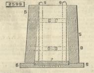
8, which are tightened by screw bolts, and can be slackened as required for expansion. Vertical iron straps 9, bolted to the sole plate 6, also assist in strengthening the mould, and are formed with eyes at their upper ends for the attachment of chains for hoisting the mould by.
