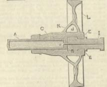
than usual to receive a split bearing E made in two halves, and forming together a round core within the hub. Recesses are formed in the core to fit collars G J and the body of the axle A, which is made holiow and contains oil. The ends I of the axle are con-nected by pins to cores E, so as to prevent them turn-ing therein, and their outer extremities fit the axle-boxes. Holes are provided to allow the oil to pass from the axle A to the bearings.
