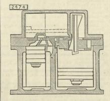
arranged to work the slide of the other cylinder. The drawing shows the arrangement.
