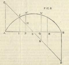
Let the curve CO cut the curve C1 D1 in J; draw JI perpendicular to AB and take OK = OI. Then as before if P lies between I and K
