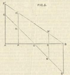
Then if the two triangles O A C and O B D are similar  $P M^1 + Q M^1 = M M^1 + M N^1$ . (26) Therefore the mean of the pressure at these two points on the
