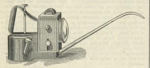
itself. It will be seen that the bull's-eye concentrates the light just where it is wanted. In the United States the can is known as the "Excelsior Illuminating Oiler," and is made by Messrs. Walker and Co., Lake-street, Chicago.
