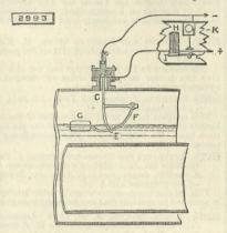
operated. The current from a generator is conducted to the water by the insulated conductor C, to which, near the low-water level, is attached a metallic surface E, kept clean and bright by the friction of a piece F, actuated by float G, when the water falls so as to be below the cleaned surface of the conductor and this circuit broken. As long as the current flows the magnet H attracts armature I, but when the circuit is broken the current is switched into a signalling apparatus K. apparatus K.
