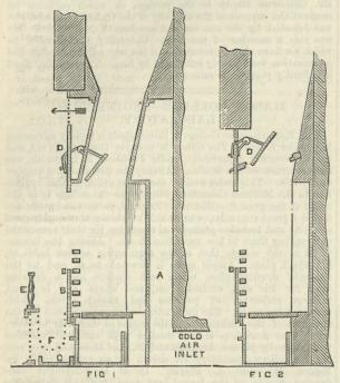
down, a blind B is suspended so as to move down by degrees in front of the body of burning fuel. A sunk ashpit is not used. The blind is balanced in front of the body of fuel by chains and weights.
