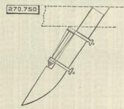
described. (2) In combination with a recessed plough-coulter, a rotary clearer having radial wings, in combi-nation with vertically adjustable supporting brackets, and with a tapering point below the wings in line with the edge, substantially as described.
