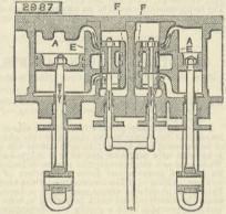
Al are arranged side by side and their pistons connected to the crank shaft, the valve chests and valves being fitted between the cylinder and separated by a partition. The valves E are operated direct from the crank shaft by a single excentric. A pair of piston valves F act as reversing valves, and their rods pass out of the valve casing and are connected so as to be operated simultaneously by one hand lever.
