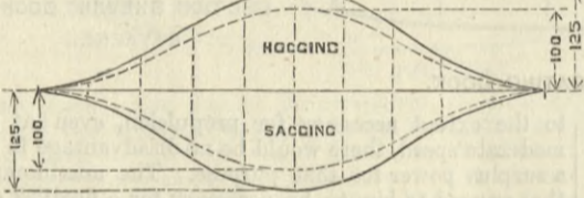
DIAGRAM OF HOGGING AND SAGGING STRAINS, TO ILLUSTRATE MR. SMITH'S PAPER, PAGE 240.
