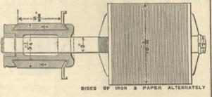
giving free access to the atmosphere, so that the temperature and resistance kept nearly constant, this resistance being almost exactly 2 ohms.
