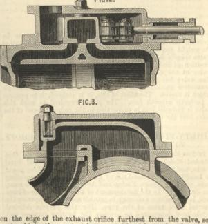
as to obtain the greatest leverage without increasing the small movement of this part of the valve.
