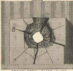
BROWN STEEL FACED PLATE AFTER IBLOW FROM 100 TON CUN STEEL PROJECTILE
