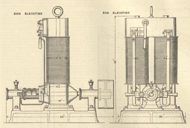
In our issue of 23rd January we shortly described a test of an Edison-Hopkinson dynamo made at the works of Messrs. Mather and Platt, of Manchester. We now give full details of this specially interesting and severe test, along with drawings of the machine.
