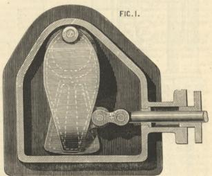
proposal aims at the root of the evil, as instead of fighting it with any kind of complicated appliance, most of which, as we pointed out, are open to break down as well as increasing the moving weight; he avoids it by removing the exhaust opening out of the line of motion and allowing the valve to partly rotate on a pivot pin placed in a position nearly or quite coinciding with the centre of the exhaust orifice. This pin is placed preferably
