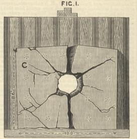
CAMMELL STEEL FACED PLATE AFTERIBLOW FROM 100 TON CUN STEEL PROJECTILE
