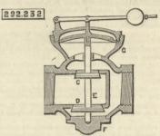
either the valve C or D, and the spider guide located between the valve C and the diaphragm G, thereby insuring the accurate seating of the valves and pre-venting the lateral movement of the diaphragm, sub-stantially as described.
