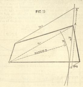
20, or 200, &c. &c. A tangent  $m_3$  to this arc is drawn from other end of  $m_1$ , and  $m_4$  and  $m_5$  are drawn  $|| m_1$ . They cut off A on  $m_3$ . The radius 2 in this construction must be least than the diagonal matrix. off A on  $m_3$ . The radius 2 in less than the diagonal  $m_1$ . The area = A, or 10 A, or 100 A, &c. &c.
