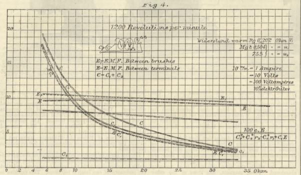
the electrical efficiency varies from 83 per cent. for R =5 ohms to 67 per cent. for R = 33 ohms. The electro-motive force between the terminals keeps very constant, being 98 volts when R = 5 ohms, and 90 volts when R = 40 ohms.
