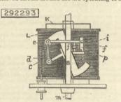
the clutch and release the earbon rod, substantially as described. (3) In an electric-arc lamp, the com-bination of the rod B, clutch f, link e, arm d, oscilla-ting armature D, and spring c, substantially as described. (4) In an electric arc lamp, the combina-tion, with the clutch f, adapted to grip and lift the carbon rod, and having fork i, of the derivation magnet K, armature L, shaft m, finger n, having forks o, cam p, having lever q, and spring r, substantially as described.
