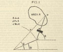
the wheel W, will be a measure of the change of the angle  $\theta$ . Let us designate this number by R. Then the change of  $\theta$  for simple rotation is  $\theta - \theta_0 = \frac{c}{m}$  R, wherein c is a constant depending on the
