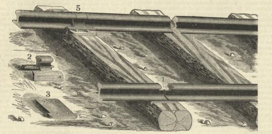
weighing from 30 lb. to 50 lb., four bolts, four nuts, and four washers, to connect the rails together; and it would appear at first sight the joints should be at least as strong if not stronger than the rail itself; but it is not, as English and American tests prove. The reason is, too many pieces constitute the joint, and these pieces cannot be screwed together so firmly—allowing for expansion and contraction—as to make them one; hence the joint is the weakest
