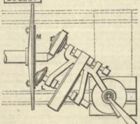
plane-faced friction wheel M, secured thereto, and the friction wheel L and its shaft, with means for transmitting the motion therefrom to the grinding wheel, as and for the purpose set forth.
