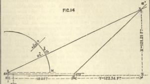
with radius O H = 5in. The line  $a^1$  is drawn parallel to O a, the angle H O a being made 43 deg. 25 min. From x the intersection of  $a^{1}$  with O b is measured X down to the ground line through station A. This is the height required. The distance Y from station A to centre of base of spire may also be directly measured from the diagram. The calculation of X by ordinary trigonometry involves the
