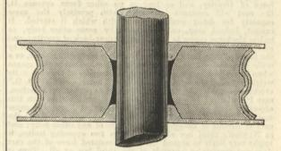
rubber within the expanding ring, and the support thus given to the rubber, without friction, reduces the wear and tear upon the most perishable part of the spring. The weight of the rubber employed in this spring is very much less than in any other previous form of the same power, and consequently
