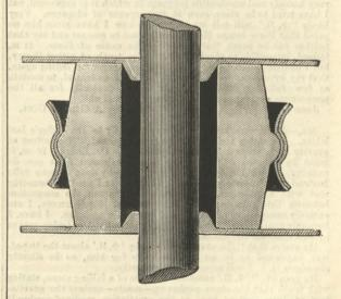
renewal is attended with proportionately less expense. The corrugated steel belt being expanded by a uniformly distributed pressure is very durable, and hence the spring, which is made by Messrs. L. Sterne and Co., Glasgow, is offered specially for buffer and draw springs for heavy mineral traffic, and for passenger vehicles fitted with continuous brakes.
