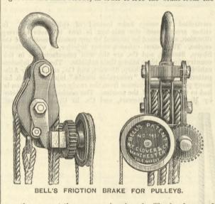
rope the moment the pressure is released. The band or cord has a turn and a-half round the pulley, which makes it unneces-sary to hold both sides of band, leaving one hand free to guide the descending weight or to hold the rope of the pulley blocks. The same firm exhibits Bell's patent low-pressure filters, as used
