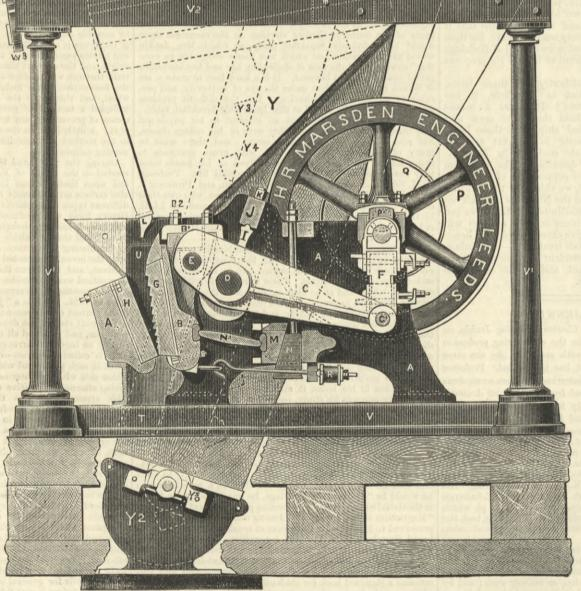
MARSDEN'S STONE CRUSHER, ELEVATOR, AND SCREEN.
