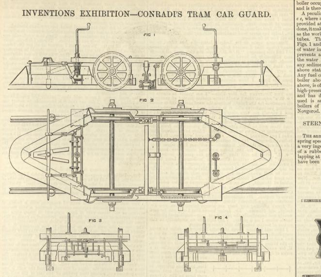
hammered in or bad rail joints. Each car is thus enabled to clear its own track. When the grooves have been sufficiently cleaned the scrapers are lifted out of the grooves by means of the lever F and chain connection. All operations are carried
