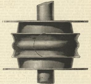
about fivefold, while the smooth action of the rubber is retained. The effect of the resistance of the belt increases as the rubber approaches the weakest point thus practically equalising the resistance throughout the entire range of the spring. There is practically no frictional movement of the
