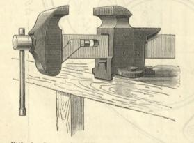
has a little freedom on the sliding bar. When it is desired to grip an object the front jaw is pulled out until it can be admitted. By slightly raising it the bar is freed from the toothed piece which holds, and it may be pulled out or pushed in. When pushed in and the jaw is touching the object, the
