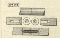
cavo-convex abutting ends, and a central flexible elastic core, securely housed in both of said rod sections, and flexibly coupling them, as set forth. (2) The combination of the rod sections, internally chambered centrally, and longitudinally connected by a non-extensible flexible link or chain, and a
