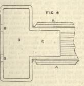
us is the adoption of a fire box shaped in plan as in the accompanying diagram. Virtually, we would have in the part C an ordinary fire-box with about 18 square feet of surface. The remaining portion D, a species of addition species of addition tacked on, so to speak, might be 7ft. by 4ft. Thus we should have a total grate surface of about 46 square feet. In
