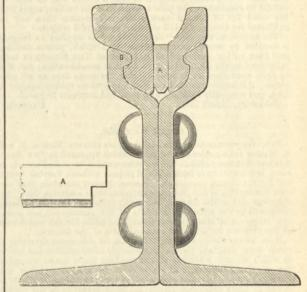
loose, and thus require a fresh set of the keys A, though if these are put in at first rather tight, so that there is initially a spring grip on the rail, looseness may not arise. The ends of the wedge strips A are notched, so as to be readily prised out of place when required. It would probably be found in practice better to make the upper face B of the angle iron parts of the per-manent way more nearly horizontal. The sleepers are laid to break joint, so that no fishing is required.
