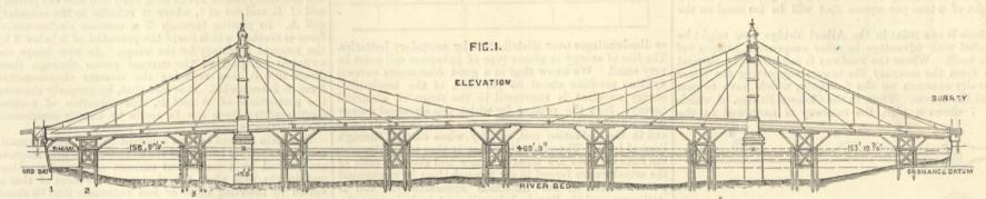
FIG. I-ELEVATION OF THE ALBERT BRIDGE SHOWING TEMPORARY PIERS.
