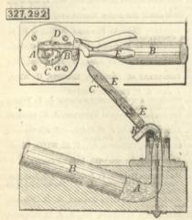
with a jaw having a rounded arc-shaped face, sub-stantially as described. (2) The combination of the bulb C or its equivalent with the annular die  $\alpha_i$  sub-stantially as and for the purpose herein set forth. (3) The combination with an annular die  $\alpha$  of a gripping or bending device for bending the metal simul
