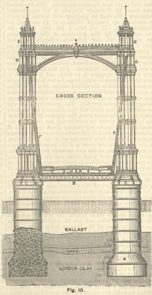
always be a certain proportion between the weight supported at the apex of the catenary and that supported by it at each of its suspending points, its form also being so calculated as to prevent any change in the proportion.
