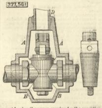
key seat having the upper opening for the reception of a turning key and the inclined openings extending a turning key and the from the said opening.
