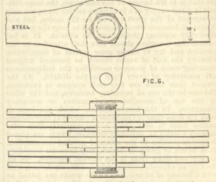
number; and in order to maintain the same sectional area of 30in., the four links are 14in. thick and the five links are 1in. thick. Assuming that the steel has a strength equal to 30 tons per square inch, the chains will have a resistance to fracture of 900 tons, or about five times the maximum strain that can in all probability be ever brought upon it.
