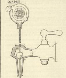
(2) A faucet having circular valve seats a surrounding (2) A nuclet naving circular valve sets a surrounding the vertical passage thereof at its junction with the horizontal passage, in combination with a ball valve seated upon the seats a and secured through its axis to a rod, as a means for operating a registering device, substantially as and for the purposes specified.
