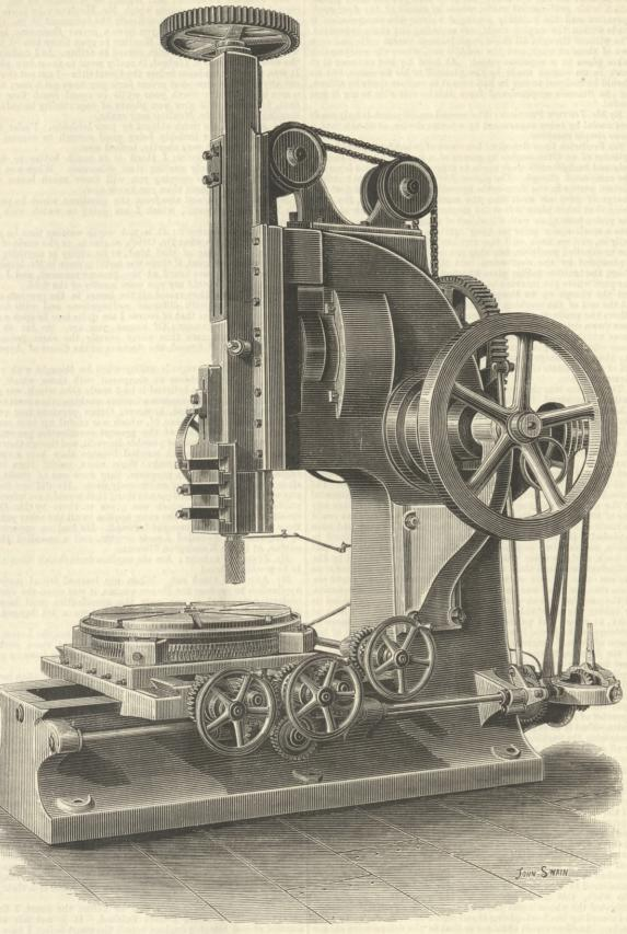
COMBINED MILLING AND SLOTTING MACHINE.
