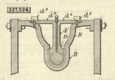
yoke B, cast in one piece, and adjustable cap D, said cap having a hollow stem  $d\lambda$ , arms  $d^2d^3$ , adjustably secured to said yoke, and flanges d, substantially as and for the purposes set forth. 327,561. Casing for STREET Cocke in Gas and WATER for the function of the fland of the fland of the fland
