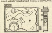
arm B<sup>1</sup>, and projection e, knob lever C, intermediate lever D, and segmental locking tumbler E, having recesses in its periphery, substantially as set forth.
