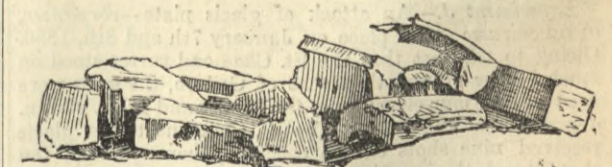
FIG 7. EARLIER PATTERN OF CHILLED IRON CUPOLA IN FINAL CONDITION OF DESTRUCTION
