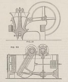
of this kind with a mouth 380 mm. by 180 mm.-15in. by 7in.running at 250 revolutions per minute, will break 6 tons of the hardest basalt per hour using 4-horse power. Huet's stone-breaker has jaws moved backwards and forwards, and at the
