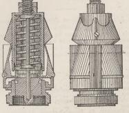
tance from the axis of the pivotted arm to the floor being less than from the axis to the lower face of the elastic pad, whereby the weight of the door will act on the arm and pad to produce sufficient friction on the floor or carpet to hold the door in any desired position, substantially as set forth.
