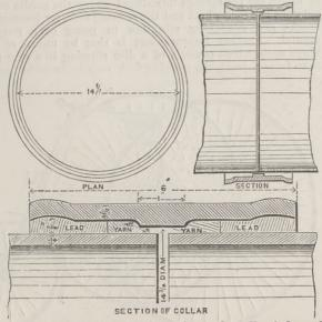
adjoining length is placed in position, the collar is brought over the joint, as shown in the sections; and the joint is caulked with yarn from both ends, over which lead is run in the ordinary way. If it be required to take up a length, the lead and yarn are picked out; and the collars of two joints are run back over the ends of the pipes, when the ength may be taken out.
