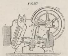
jaw by the plate B. The return motion of the movable jaw is given by a rod and lever, and is equalised by rubber buffer W. A machine of this kind, with the mouth 200 mm. by 380 mm. —8in. by 15in.—running at 250 revolutions per minute, will break 6 tons of the hardest baselt, to what size in the size of the second break 6 tons of the hardest basalt-to what size is not given-
