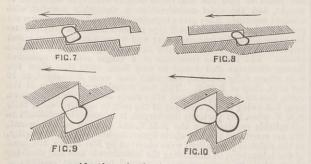
same, on one side there is the internal friction of the smallest particles of the body in opposition to the regular transmission of the force; the friction of the crushed body on the surfaces hinders the movement of the same along these surfaces. According to Kick's researches (*Dingler's Poly. Journ.*, 1877, vol. 224, p. 465) the particles form into sliding cones, supporting
