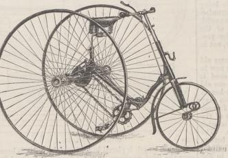
its normal position, as shown in the engraving, to the vertical, for permitting a lady to mount without soiling her dress against the wheels, the fork being afterwards securely locked in position by a bolt, rod, and handle. For lady's use also the chain is enclosed in a light guard of wire gauze. The brake is controlled by hand or foot at option, and all working parts except the pedals are fitted with the adjustable ball bearings described and illustrated below
