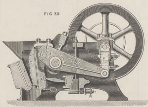
on the strong bolt D, the friction is reduced by the link I, the lever C takes hold of the jaw B by the bolt E, and gives it a kind of circular motion; the jaw B is supported against a toggle resting against an adjustable block; a complex up-and down to-and-fro motion is thus given to the jaw B. A machine
