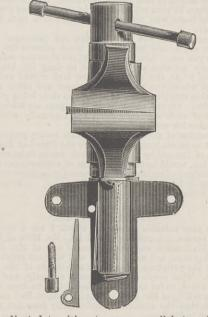
the vice adjusted to either taper or parallel, to suit work in hand. The screw is boxed up, so that no filings can fall into it. The vice has been put together for strength and durability, the jaws and body being made solid from best Yorkshire wrought iron.
