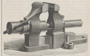
parallel vices, combined with greater strength in the eye—which is the weak place in most parallel vices—and the special advan-tage of a taper grip, by which any taper article is held with the greatest firmness and without the possibility of slipping. This grip is obtained by simply removing a wedge on the right-hand side of the vice, which can be done in a couple of seconds, and
