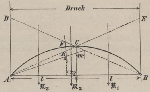
$$R_3 < \frac{l - x_2}{x_2 + m} \left( R_1 \frac{m}{l} + R_2 \right) \dots \dots \dots (58)$$
