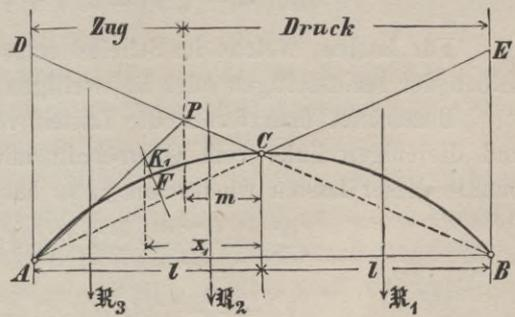
$$R_2 < R_1 \frac{m}{l} \dots \dots \dots (59)$$
