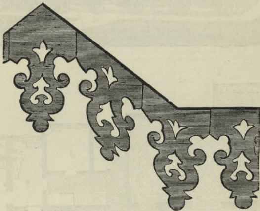
French cut pine woodwork, from the exterior.
