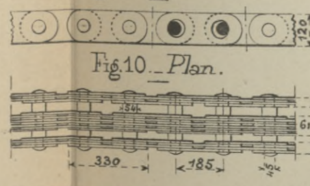
Chânes de suspension. Echelle: (\frac{1}{20}) 0,05 p.m. Fig. 9. Elevation.
