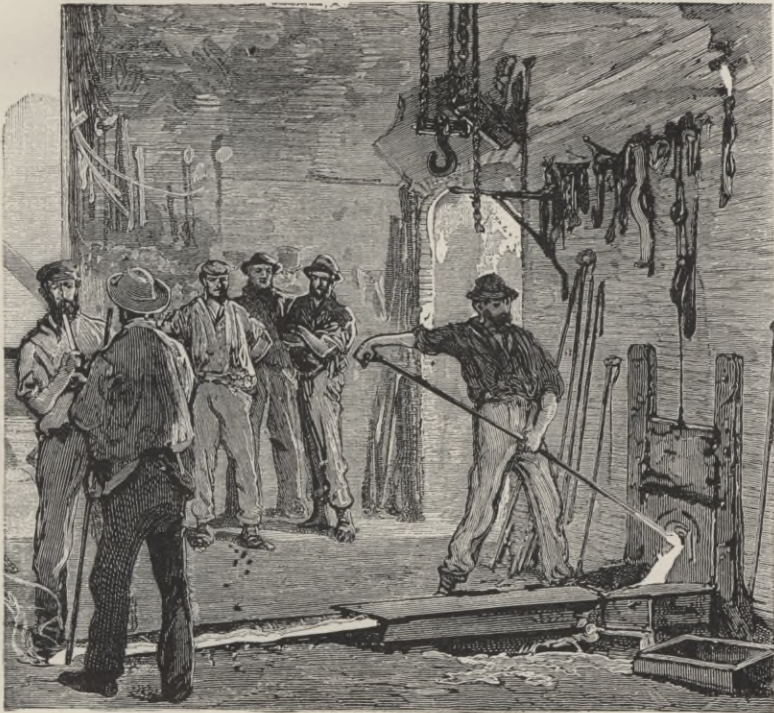
Fig. 33. Running melted bronze (an alloy of copper, zinc, and tin) from the furnace to the mold.
