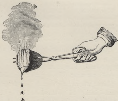
Fig. 65. When metallic zinc is heated, it melts, vaporizes, and oxidizes (affording flame, and producing a white smoke composed of solid particles of zinc oxide, \text{ZnO} ).
