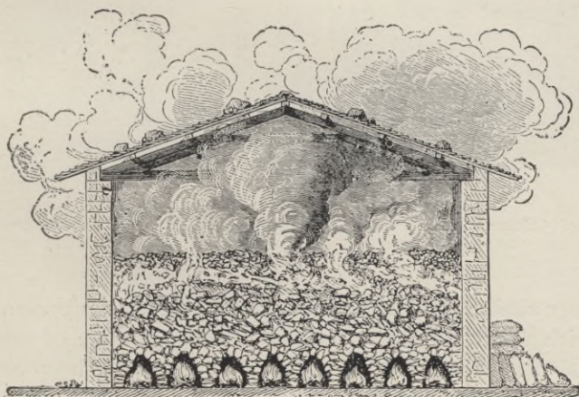
Fig. 59. Hydrated calcium sulphate, when heated, loses its water, plaster of Paris remaining.
