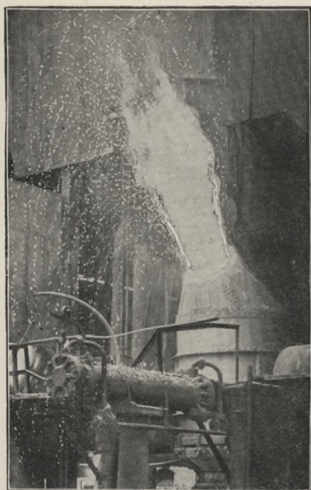
Fig. 93. View of Bessemer converter during the blow; the cylindrical object in the lower foreground is part of the hydraulic apparatus for turning the converter upon its axis.
