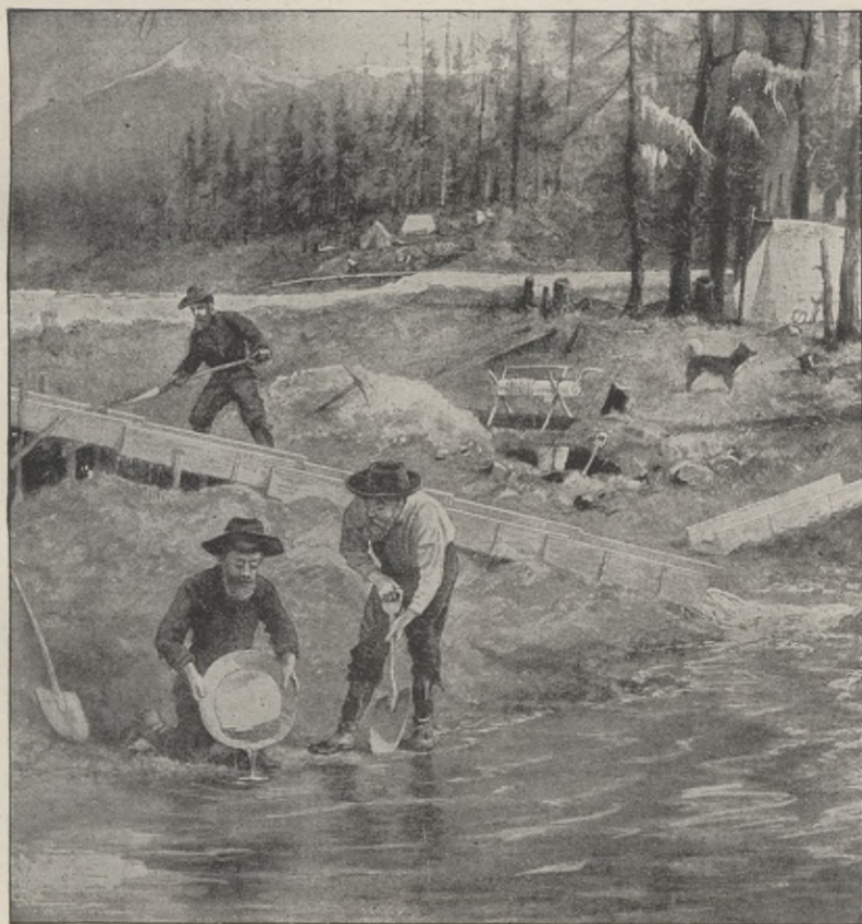
Fig. 46. Sluice for washing auriferous earth in placer mining. (The men in the foreground are testing the earth by "panning.")
