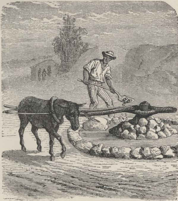
Fig. 34. Arrastra, used in the first stages of the Mexican process, for pulverizing silver ore.
