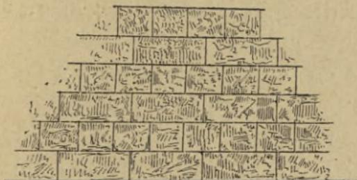
FIG. 14. — APPAREIL RECTILIGNE.
