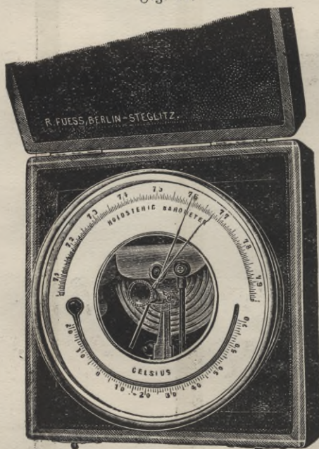
Stations-Aneroid-Barometer. ca. \frac{1}{3} n. G.
