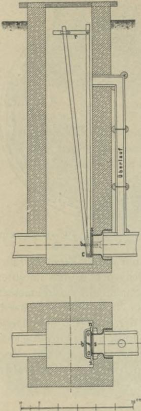
Fig. 327. Wodick's Ventildrainage.
