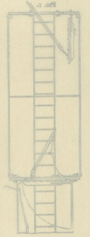
FIG. 1.—VERTICAL SECTION THROUGH AIR-LOCK AND MAIN SHAFT.
