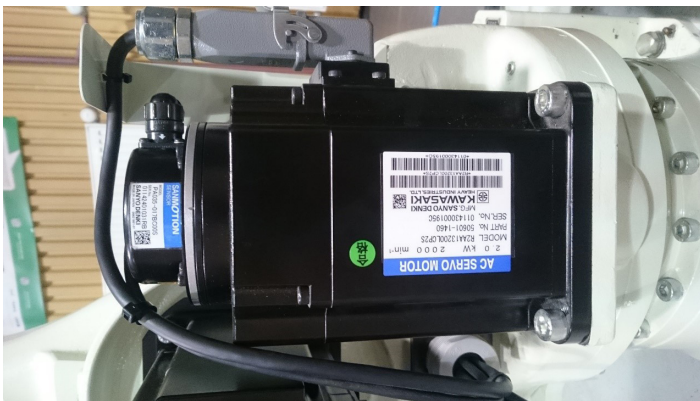
Fig. 3. Applied motor with absolute encoder
