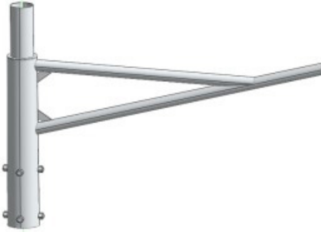
Fig. 16. Strengthening the structure in the place where the light arm boom is connected to the supporting structure of the column
