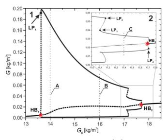
Fig. 2. Bifurcation diagram for value of dilution rate  $D = 0.1000 [h^{-1}]$  relative to feed stream glucose concentration  $G_0$ ; A –  $G_0 = 14.0 [kg/m^3]$ , B –  $G_0 = 16.0 [kg/m^3]$ , C –  $G_0 = 17.4 [kg/m^3]$
