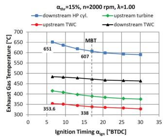
Fig. 17. Exhaust gas temperature of the five-stroke engine as a function of the ignition timing
