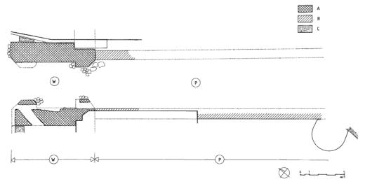
Fig. 14. Kożuchów, Głogowska Gate, projection of fundaments with chronological wall stratification. A – 1st half of 14th century; B – 2nd half of 14th/1st half of 15th century; C – 18th century; W – tower, P – foregate; reconstruction lines – dotted (drawn by A. Legendziewicz)
