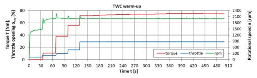
Fig. 22. Conditions for conducting the test of warming up the TWC with a ceramic support
