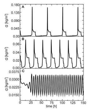
Fig. 3. Time trajectories of glucose concentrations (*G*); A –  $G_0 = 14.0 \text{ [kg/m^3]}$ ,  $D = 0.1000 \text{ [h}^{-1]}$ ; B –  $G_0 = 16.0 \text{ [kg/m^3]}$ ,  $D = 0.1000 \text{ [h}^{-1]}$ ; C –  $G_0 = 17.4 \text{ [kg/m^3]}$ ,  $D = 0.1000 \text{ [h}^{-1]}$
