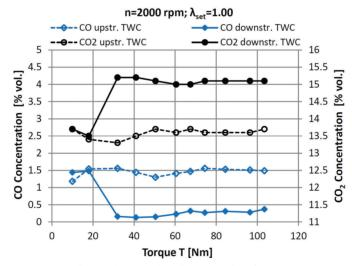
Fig. 9. Volume concentration of CO and  $CO_2$  in the exhaust gas of the five-stroke engine co-operating with a catalytic converter with a ceramic support as a function of the engine load
