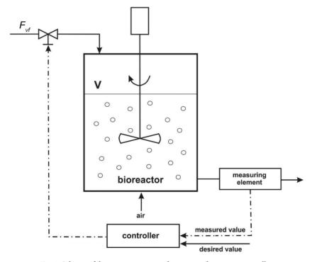
Fig. 1. Scheme of the process system with automatic bioreactor controller
