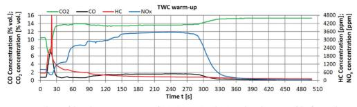
Fig. 24. Charts of the volume concentration of CO, CO<sub>2</sub>, HC and NO<sub>x</sub> in the exhaust gas of the five-stroke engine during the test of the process of warming-up the TWC with a ceramic support
