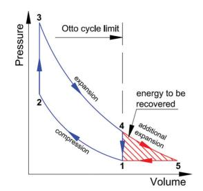
Fig. 1. Otto cycle with the marked area of work of additional expansion
