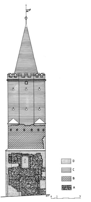
Fig. 21. Prudnik, Dolna Gate's tower, north elevation with chronological wall stratification. A – 1st half of 14th century; B – 2nd half of 15th century; C – around 1580; D – 19th and 20th centuries (drawn by A. Legendziewicz)
