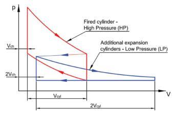
Fig. 3. The basic theoretical cycle of the fired cylinder (red line) and the cycle of additional expansion conducted in a separate cylinder (blue line)
