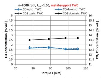
Fig. 20. Volume concentration of carbon monoxide and carbon dioxide in exhaust gases of a five-stroke engine co-operating with the converter with a metal support depending on the load
