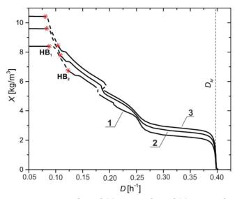
Fig. 4. Bifurcation diagram for  $G_0 = 14.0 [kg/m^3] (1)$ ,  $G_0 = 16.0 [kg/m^3] (2)$ ,  $G_0 = 17.4 [kg/m^3] (3)$ , relative to dilution rate D, made to determine the value of critical dilution rate  $D_{tr}$ .
