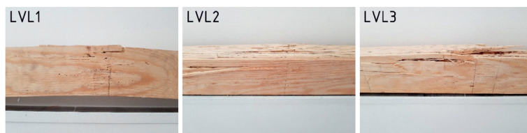
Fig. 3. Failure modes of reference beams
