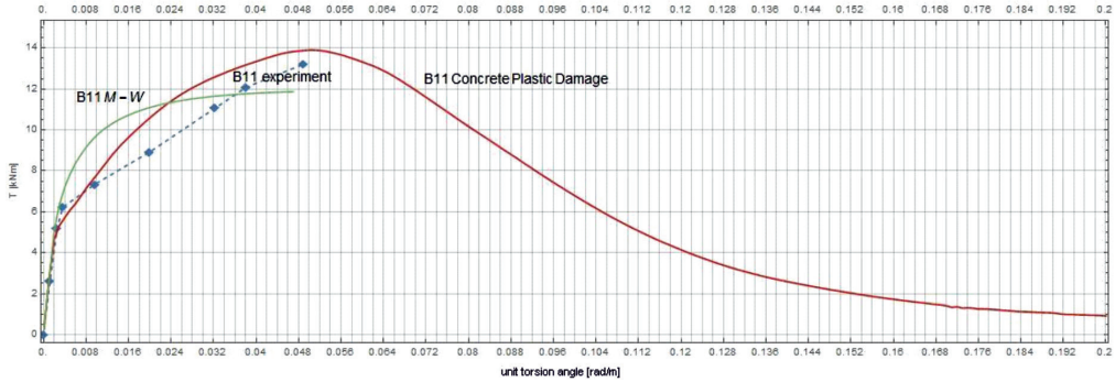
Fig. 9. Torsional moment – unit torsion angle relationship for beam No. B11 for Concrete Plastic Damage and M-W material models
