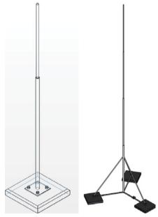
Fig. 1. View of cantilevered mast MA4-4m (a) and tripod mast MAT6-6m (b)
