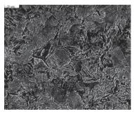
Fig. 5. Bainite microstructure
