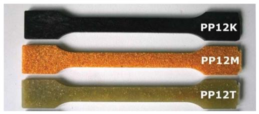
Fig. 1. Injection moulded samples with ground coffee grains, wood flour and tuff
