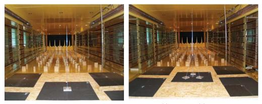
Fig. 4.Models of the masts: cantilevered (a) and tripod (b) in the wind tunnel working section
