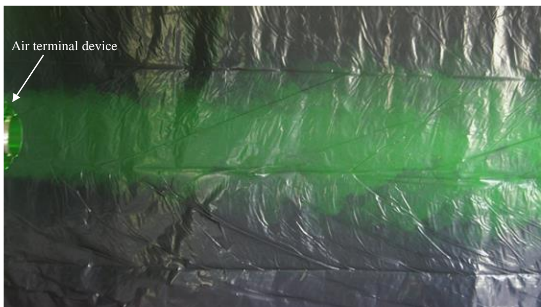
Figure 41. Laser measurement of the airflow.
