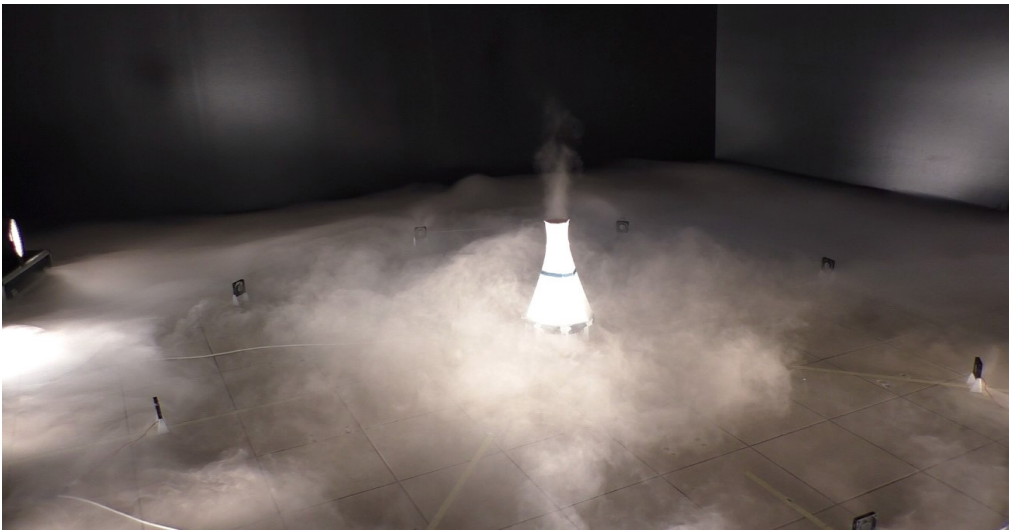
Fig. 7. Moment of turning on the system showing a visible circular gap in the fog forming due to the air movement
