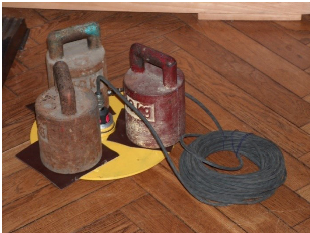
Fig. 3. Old version of measuring disc with three additional weights
