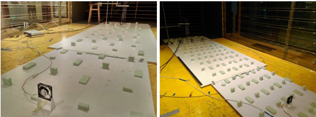
Fig. 7. Styrofoam blocks glued to the board in a pattern recreating terrain roughness for the scale model for categories III (forests and suburban areas) (a) and IV (downtown urban areas) (b) according to [25]
